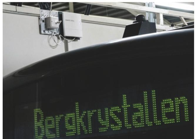
With the SIMATIC RTLS gateways, the position of the vehicles is captured to within a few centimeters.
