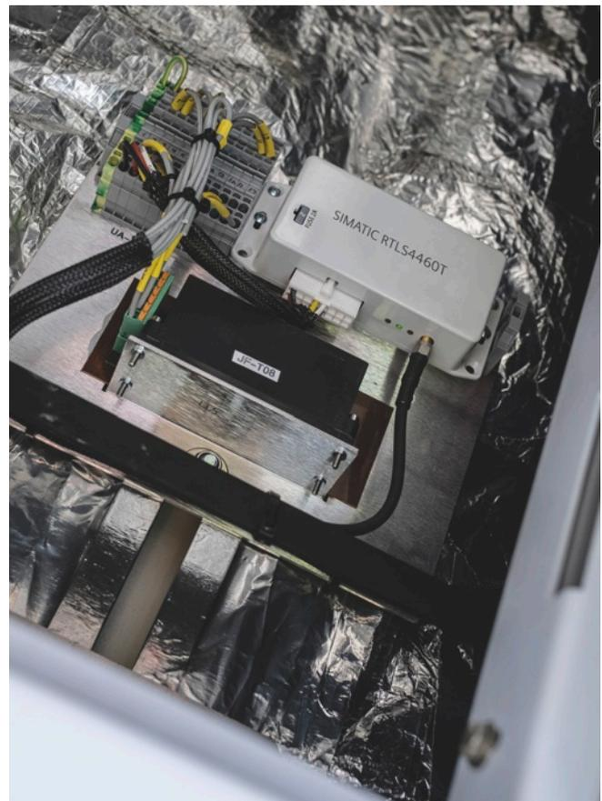
The RTLS transponders also transmit other information from the vehicles (direction of travel, coupling status).
