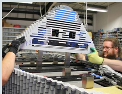
For safety reasons, Bright Bricks installs an interior steel structure to stabilize larger models
