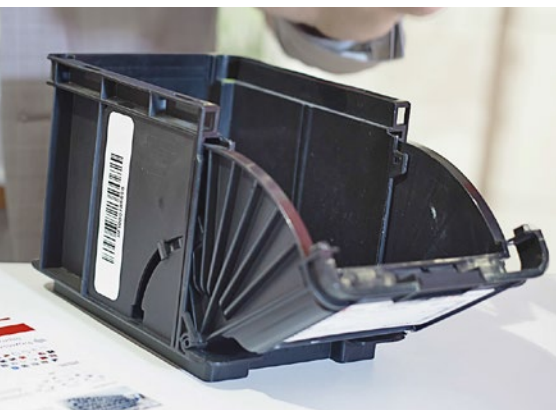
Data transferred to the central warehouse several times a day by inconspicuous iBoxes automatically trigger ordering processes based on consumption
