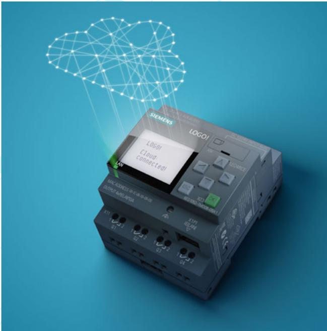
To solve small automation tasks as simple as possible is the goal of the logic module LOGO!. With this proposition, the new version 8.3 of the controller LOGO! will feature a cloud connection. The cloud connection offers even more options for centrally controlling and analyzing multiple machines or applications independent of location.
