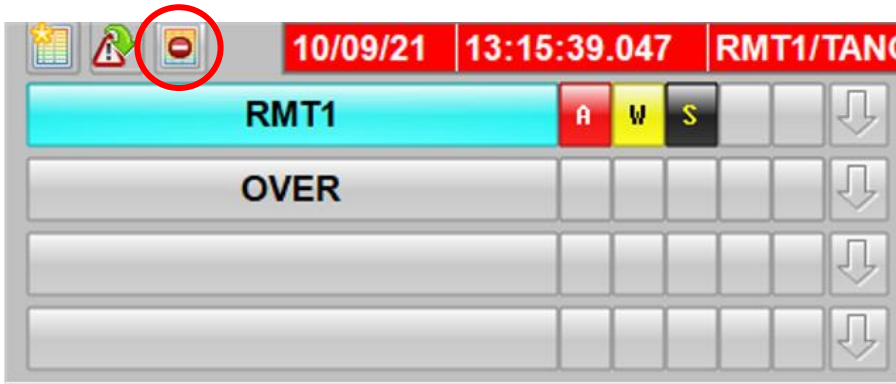
Figure 8 – Active icon indicating that hidden alarms exist (circled in red)
