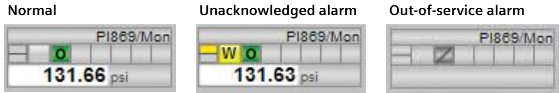
Figure 5 – Alarm state indications in symbols
