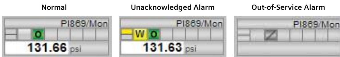
Figure 5 – Alarm state indications in symbols
