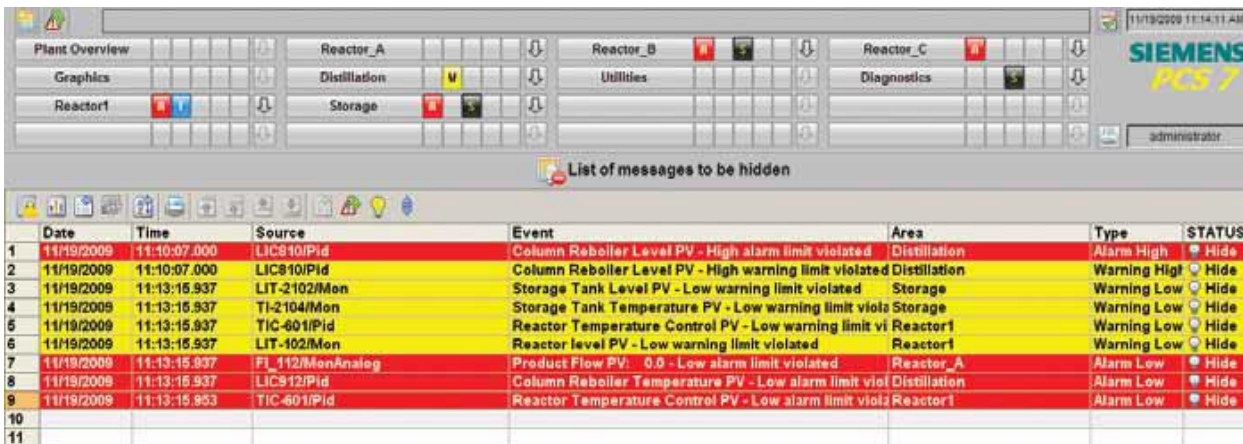
Figure 7 – HMI list of shelved alarms
