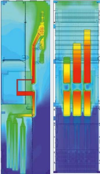
Temperature rise in circuit-breaker cubicle without forced cooling
