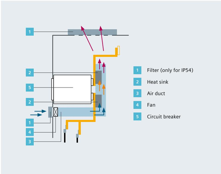
Forced cooling for circuit-breaker design
