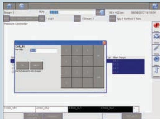
The display also supports the use of pop-up dialog boxes for entering data and providing additional operational information when needed.
