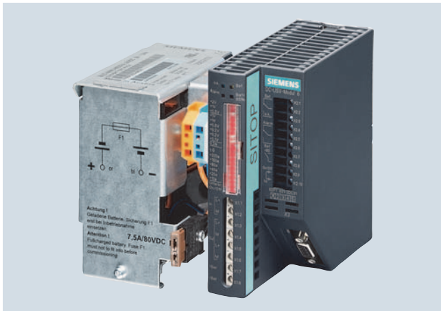
Configuration with SITOP DC UPS and battery module: 24 V buffering to maintain communication, signaling and sensor measured values. To relieve the load on the UPS, the actuators are supplied directly from the power supply unit.
