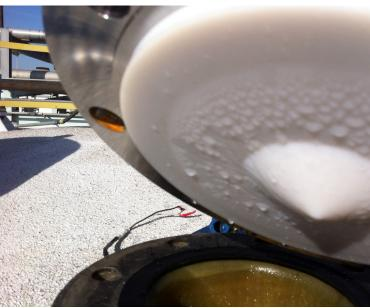
Droplets of chemical form over time on the transmitter's lens, but did not affect the SITRANS LR250's performance in any way.
