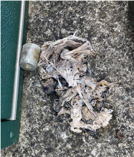
Image of clogged material from a sewage pumping station in the Yorkshire Water network, following an alert by SAM4 Health’s clogging detection feature:
