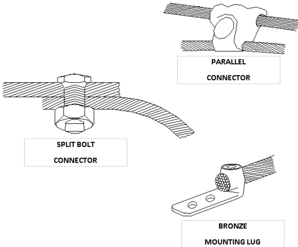
**Figure C-4 Typical Connections for Grounding and Bonding**
