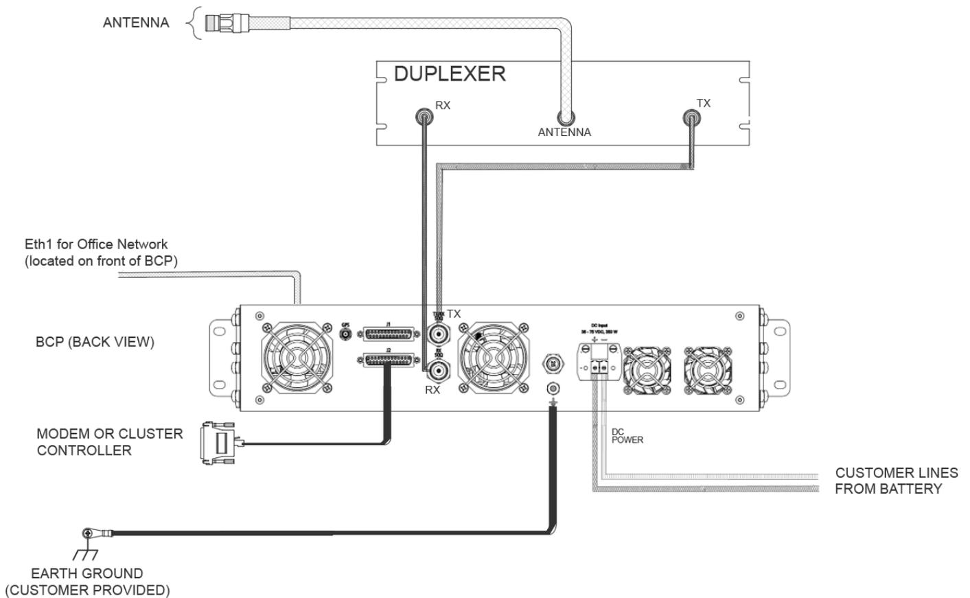
Figure 4-11 Airlink BCP Typical Interconnect Diagram with Duplexer
