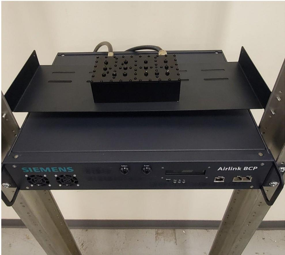
Figure 4-6 Duplexer and Airlink BCP Front Views when Mounted to Rack
