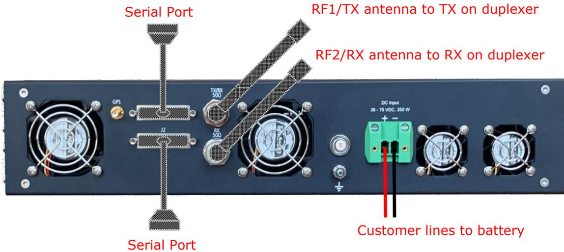
Figure 4-10 Airlink BCP Typical Interconnect Diagram – Back view
