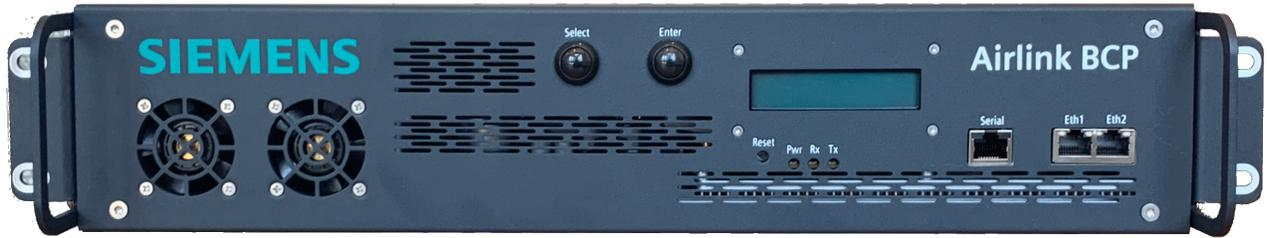
**Figure 1-2 Airlink Base Communications Package (BCP) – Front View**
