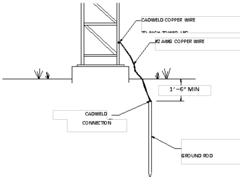
Figure C-3 Typical Tower and Pole Ground Connections
