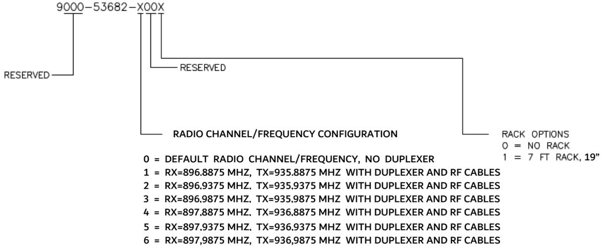
Figure 1-5 Airlink BCP Configuration Chart
