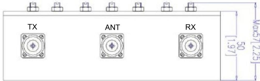
Figure 3-5 Outline Diagram of Anatech Electronics AE897-936DB5521 Duplexer
