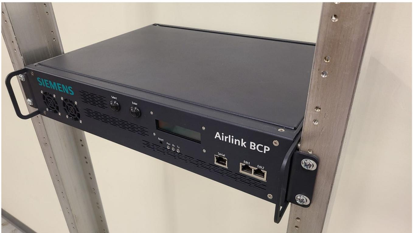
**Figure 4-2 Airlink BCP Top/Front View when Mounted to Rack**
