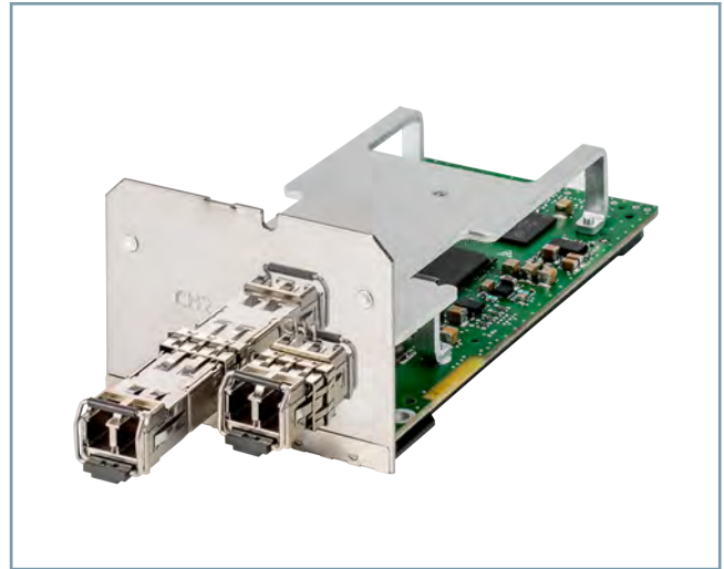
Figure 3.7/7 Optical Ethernet Module (ETH-BD-2FO)
