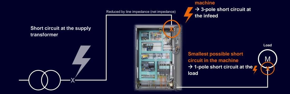
The manufacturer has to ensure, that all assembled protections devices in the machine can disconnect the highest and lowest short circuit safe!
