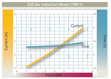
The graphs show the different point machine models' ability to handle various loads; illustrated is the typical relationship between current draw (A), motoring time (s) and load force (kN). A polynomial trend line was used to get a smooth curve.
