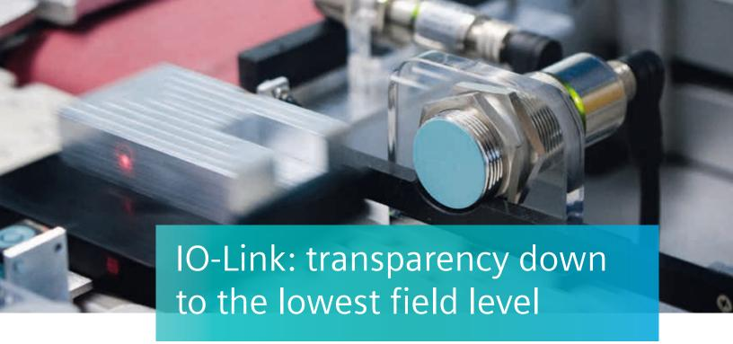
The top priority in industry is to reduce costs, increase machine and plant availability, and ensure maximum quality. One key factor: uninterrupted transparency, down to the last meter. This is precisely what IO-Link is for, an open communication standard that can be integrated in all common fieldbus and automation systems.
