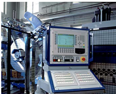
Figure 10-8 Example of operator station with EMERGENCY STOP
