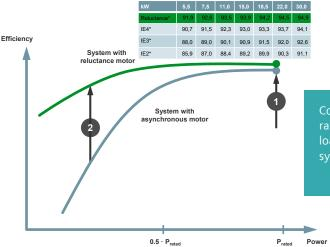
Comparison of energy efficiency at the rated operating point and in the partial load range for an induction motor and a synchronous reluctance motor
