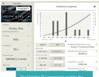
The Simotics EE Comparator enables the comparison of different low-voltage motors
