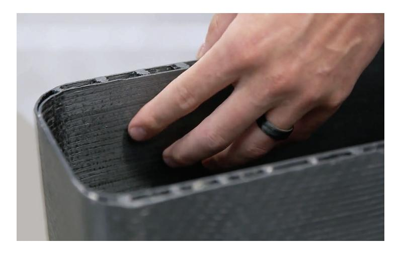
Bischoff explains that the tape is deposited quickly, establishing the form. Next, the support material additive is then completely dissolved away, leaving behind a component in the exact shape the manufacturer needs.
