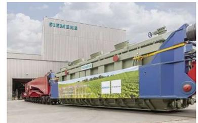
The 420 kV power transformer with a rated power of 400 MVA in the test bay and during delivery.
