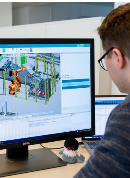
BSH uses simulation software like Process Simulate to simulate manufacturing processes and the interaction between robots and humans, including ergonomics.
