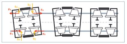
Fig. 11: Operating principle of the longitudinal drive when bogie is misaligned in the track  $S_y$ : Geometrical profile forces in y direction
