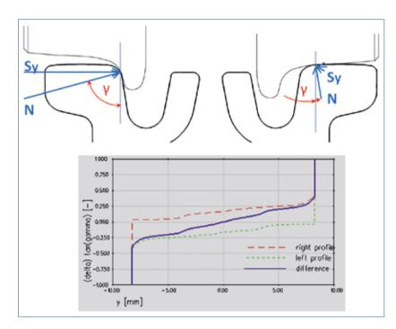
Fig. 5: Balance of forces on laterally offset pair of single wheels N: Normal force in the contact surface  $S_y$ : Geometrical profile forces in y direction  $\gamma$ : Contact surface inclination delta tan(gamma): Centering factor
