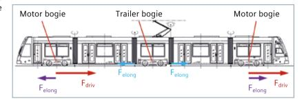
Fig. 12: Principle of "vehicle stretching" to support the centering of the trailer bogie, using the example of the Avenio M
