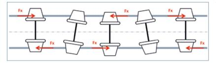
Fig. 4: Hunting motion of the wheel set  $F_x$ : Longitudinal friction force
