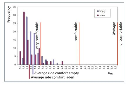
Fig. 15: Frequency distribution of the  $N_{\text{MV}}$  characteristics according to EN 12299 in the ride comfort measurements of the Avenio Munich
