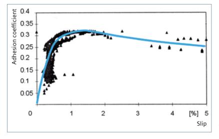
Fig. 9: Friction force slip function for the longitudinal direction according to a measurement determined by Deutsche Bahn (Source [5])
