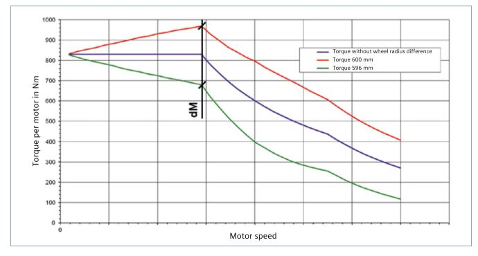
Fig. 10: Torque-speed characteristic of the Avenio motors when controlled via a common traction converter with or without wheel radius differences at the contact points
