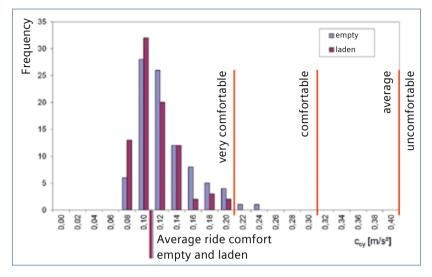
Fig. 14: Frequency distribution of the  $C_{cy}$  characteristics according to EN 12299 in the ride comfort measurements of the Avenio Munich
