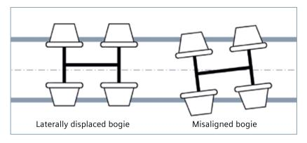
Fig. 1: Possible incorrect positions of the running gear on the track
