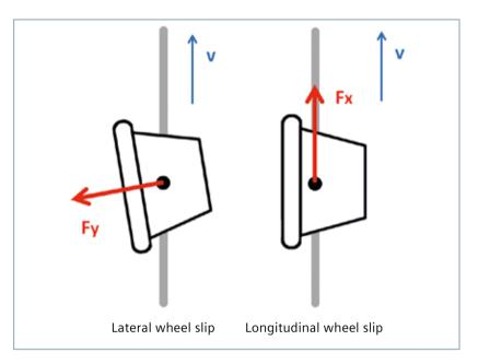
Fig. 2: Friction forces in transverse and longitudinal direction at the wheel/rail contact point v: Running speed
