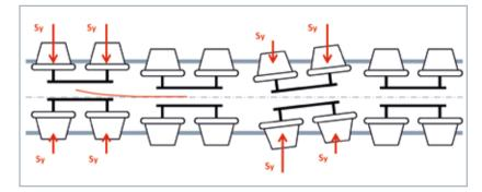
Fig. 6: Release of IRW from lateral offset and misalignment due to geometrical profile forces  $S_{\rm V}$ : Geometrical profile forces in y direction
