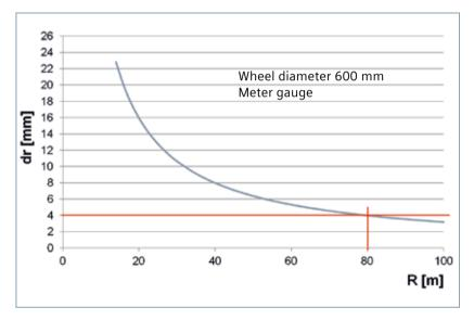
Fig. 8: Wheel radius difference that is necessary for rolling free from longitudinal slip, in relation to curve radius.
