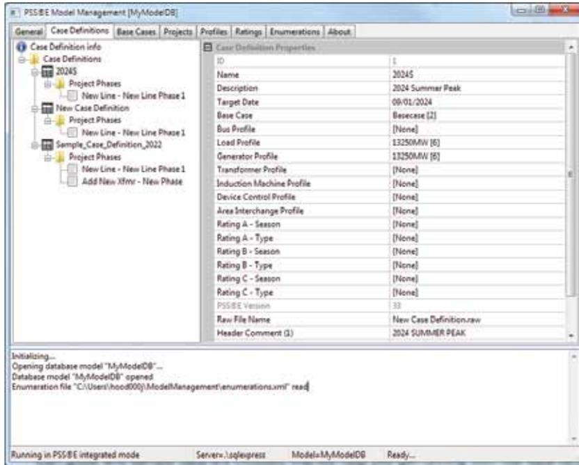
The main Model Management Module user interface. Simply select a pre-defined case definition, and a case will automatically be built from a combination of projects and generation/load profiles.
