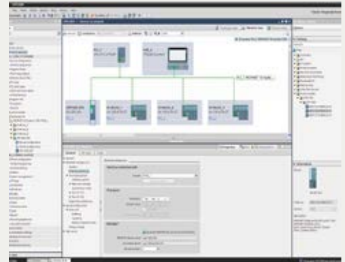
Integrating the SITOP UPS1600 DC UPS into PROFINET is easy and fail-safe via the TIA Portal.
