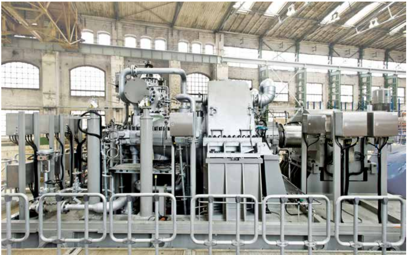
Figure 9: First Enhanced Platform steam turbine in manufacturing.
