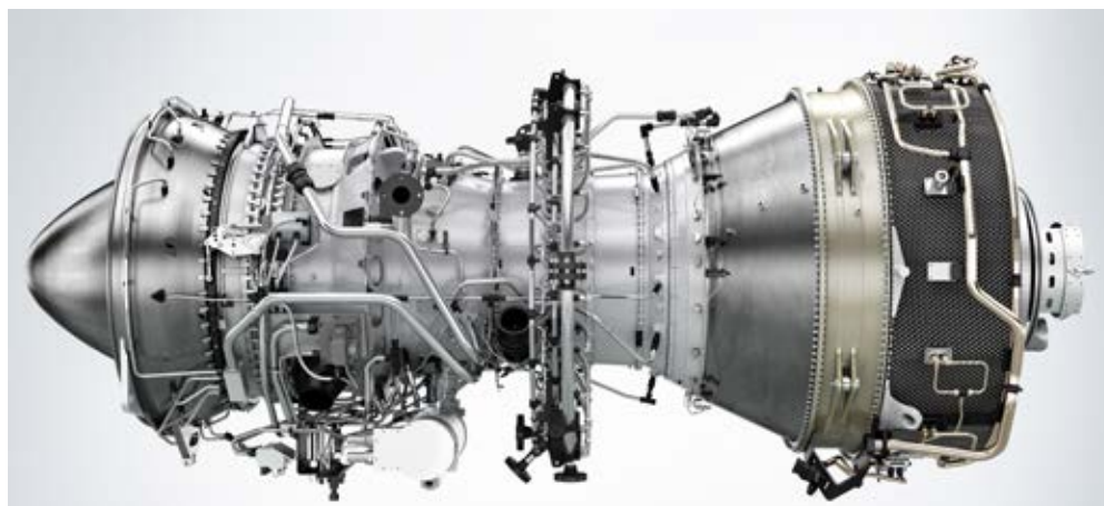
45-MW class core engine derived from the Industrial Trent 60
