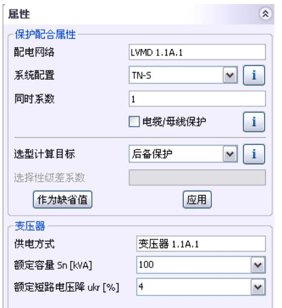
The screenshot shows both the 'Protection Cooperation Properties' and 'Transformer' sections of the Properties dialog. The 'Transformer' section contains fields for: 供电方式 (变压器 1.1A.1), 额定容量 Sn [kVA] (100), and 额定短路电压降 ukr [%] (4).
