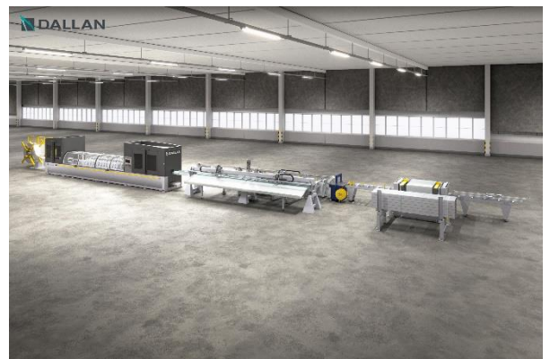
The new 'FULL ELECTRIC punching, roll forming, and cutting system', shown here with a packaging module, is Dallan's answer to the question of what the future of strip processing should look like.
