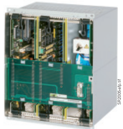
Fig. 13/64 SIMEAS R, front view. A DAU can be seen in the middle slot
