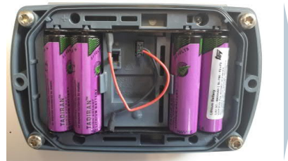
Connect battery plug
