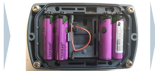
Open CONNECT 400 housing cover
