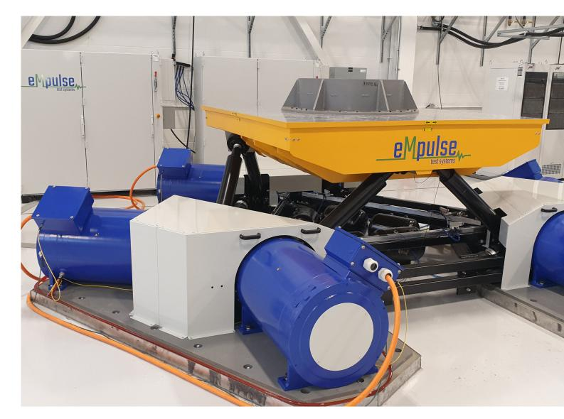
As the company's CTO, Boals offers his view on the Siemens portfolio and technologies: "Siemens has a wide range available hardware which lets us easily size our road simulators and seaMast systems to a customer's specific application requirements. Our own eMpulse proprietary configurations enable us to increase the performance of our servo-electric actuators far beyond what other suppliers' servomotors can deliver. This allows eMpulse to offer unique durability and endurance testing solutions."
