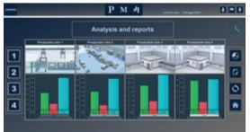
WinCC Web Navigator and WinCC WebUX are mechanisms to provide remote information access. Web Navigator is the earlier platform and interfaces using Microsoft Internet Explorer. It permits mobile control along with data analysis. WebUX (User Experience) is a newer tool more aimed at reporting. It can operate with any browser and any type of device using HTML 5.
