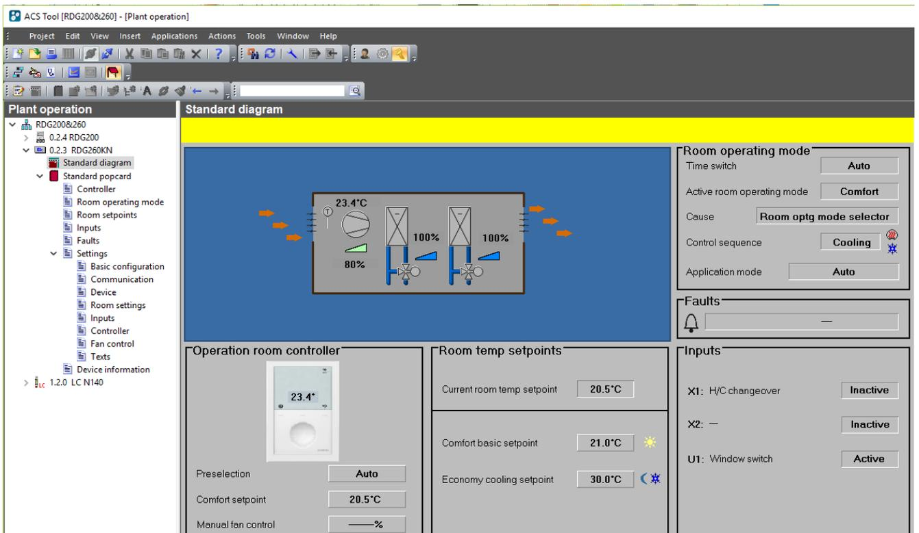
The ACS tool provides standard plant diagrams for RDG2..KN room thermostats, depending on the following configuration:
