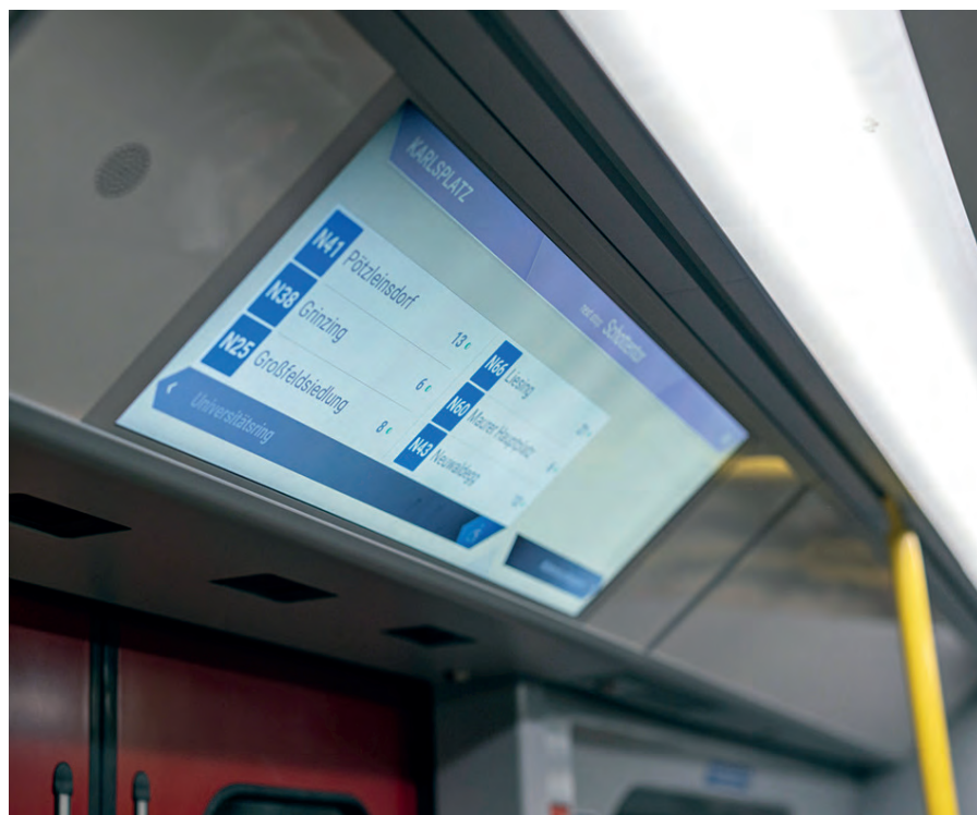
Figure 7: PI+ monitor: Monitor for displaying Passenger Information Plus content above each passenger door
