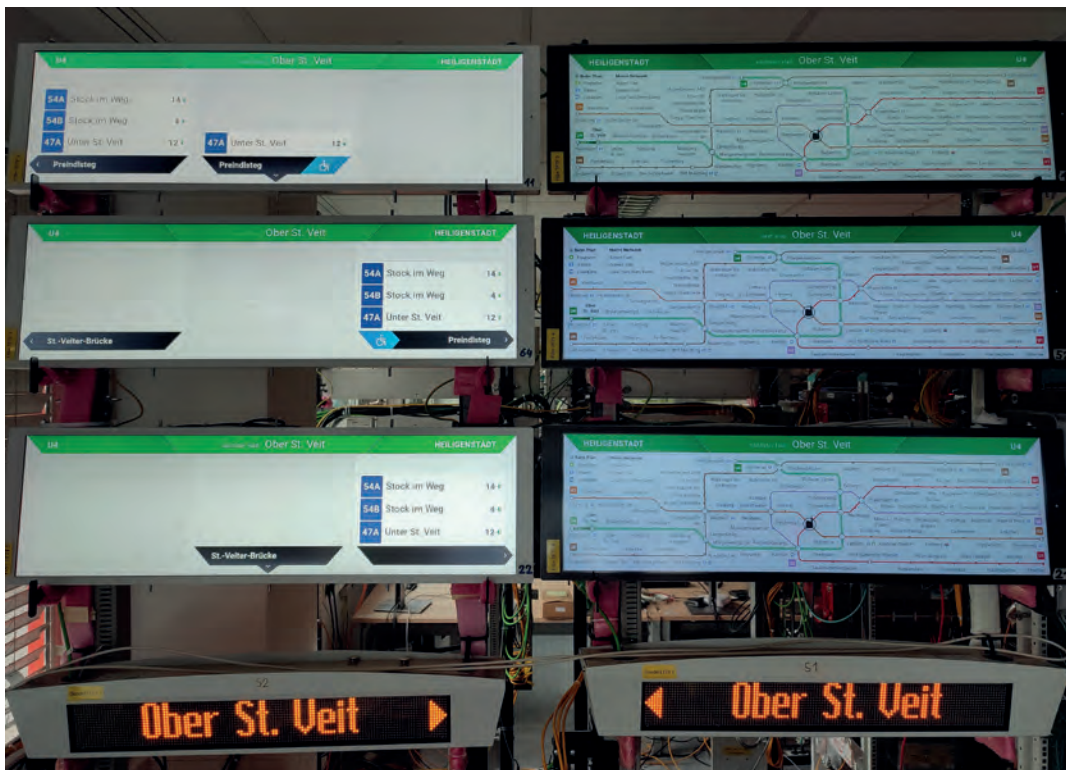
Figure 10: PI+ Laboratory configuration: Passenger Information Plus test setup in Siemens Mobility’s software laboratory
