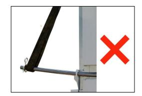
Fig. 38: Heavy weight sling attached incorrectly
