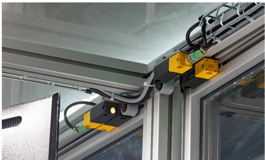
Figure 2 (optional) The non-contacting RFID safety switches with maximum protection against manipulation (3SE63) ensure that the doors of the plant are reliably monitored. Source: Siemens AG
