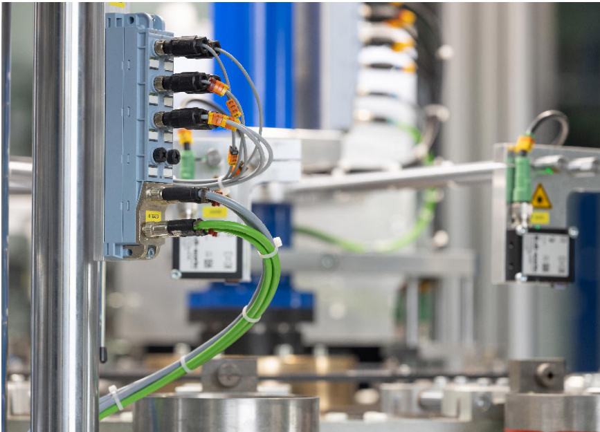
Figure 3 The scalable and highly flexible Simatic ET 200AL distributed I/O system is used to connect the process signals to a higher-level control system via a fieldbus.
