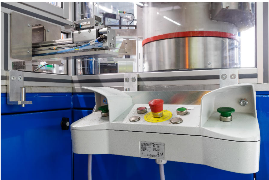
Figure 4 Two hand control equipped with pushbuttons and indicator lights Sirius Act guarantees a safe operation of the machine. Source: Siemens AG
