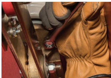
Figure 43: Loosen casting mounting bolts
