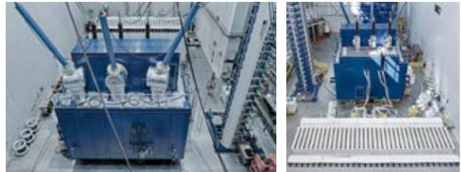
Power transformer with ester insulation and heat exchanging device in the testfield
