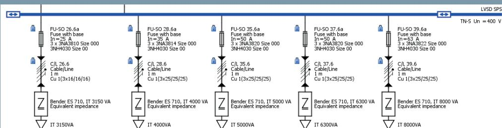
Figure 3: Cable cross-sections and backup fuses for IT isolating transformers
