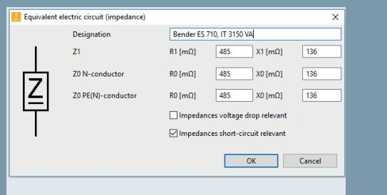
Figure 2: Entering resistances and reactances for the equivalent impedance
