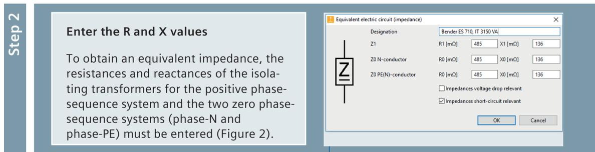
Figure 2: Entering resistances and reactances for the equivalent impedance
