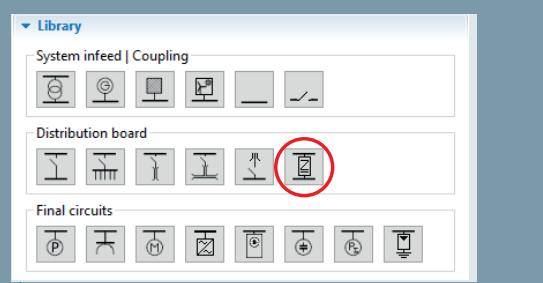
Figure 1: Adding the equivalent impedance
