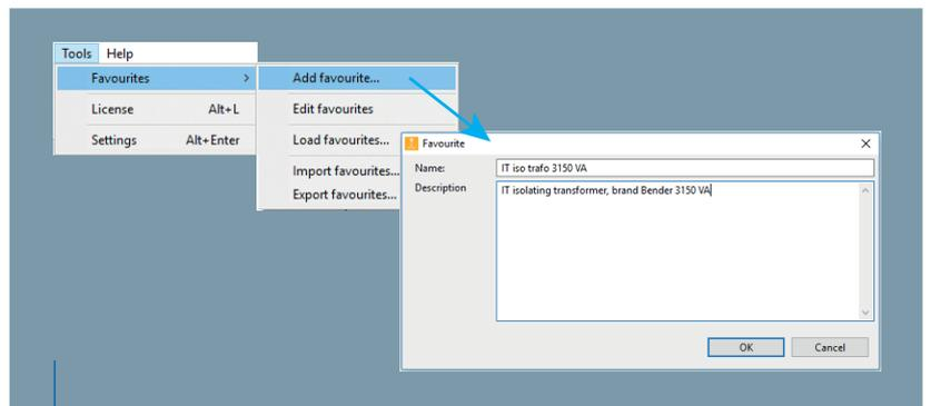
Figure 4: Context menu of the subdistribution board with equivalent impedance and input dialog for saving as Favourite
