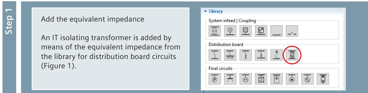
Figure 1: Adding the equivalent impedance
