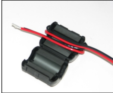
Figure 2-5 EMI Filter Installation (Showing Wire Loops)
