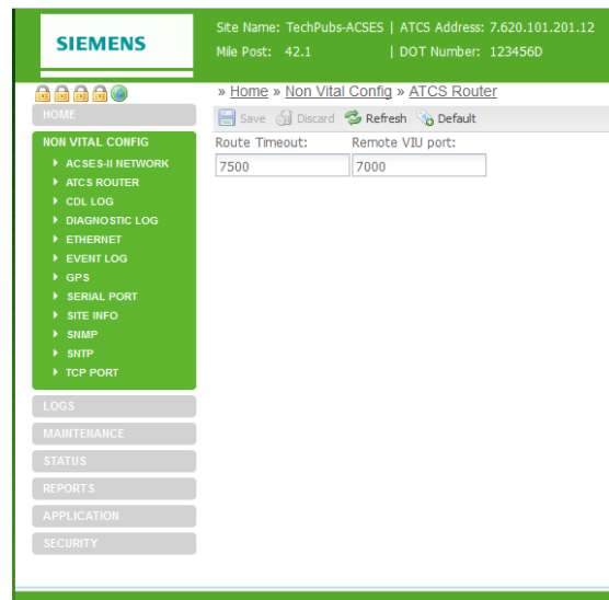
Figure 7-20 ATCS Router Configuration Screen
