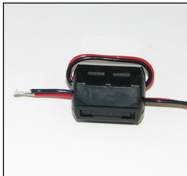
Figure 2-6 EMI Filter Installed
