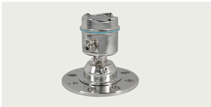
Figure 2 - Modern high frequency radar with Process Intelligence, narrow beam angle, and aiming capability that to provide reliable level measurement in dusty bins with steep angles of repose, obstructions in the silo, and deep bottom cones.
