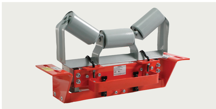
Figure 5 – Belt scales measure solid bulk material as it is transported by conveyor belt. Belt scales that use parallelogram load cells remove horizontal forces without the need for pivots allowing easier installation.
