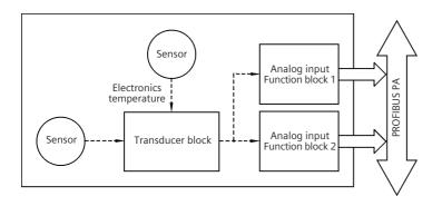
The sensor information is fed into a transducer block, which then sends information into analog input function blocks. Note that the analog blocks are called *input* blocks because the information flow is from the control system's point of view. These analog input blocks are similar to the analog input blocks for a 4–20 mA input except that, in this case, they do not run in the main controller and they provide status information as well.
