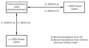
PROFIBUS and PROFINET International PI has published guidelines<sup>3</sup> on cable separation. These recommendations may be different from the local regulations. For example, in the diagram above, the recommendations from PI and from the Ontario Electrical Safety Code<sup>4</sup> for two different levels of power cables are compared, and they are dif-
