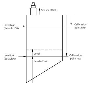
Built into the profile is a definition of the output and a method for scaling. The scaling is done in the device by using an analog input block, called *input* because the data is viewed from the PROFIBUS master perspective. The output of this block consists of IEEE floating representation of the process variable plus a status byte.
