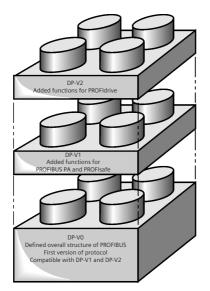
The second version of the PROFIBUS DP specification, DP-V1, added functions for process automation and safety application (PROFIBUS PA and PROFIsafe), and used the same overall command structure as defined in DP-V0 while ensuring interoperability. Interoperability is the ability to take any vendor's device, connect it to a PROFIBUS network, and have it work.
