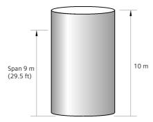
Define the range of the application in the level calibration block of the transducer block using the information from the block diagram.
