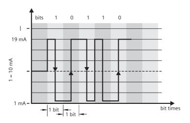
The voltage level on the bus has to be a minimum of 9 V DC,<sup>4</sup> but can be as high as 32 V DC. The baud rate is fixed at 31.25 Kbits/second. This is the main physical layer used for PROFIBUS PA.
