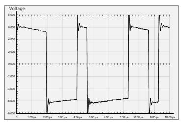
Small PROFIBUS DP network running at 1.5 meg with no terminators and with some communications
