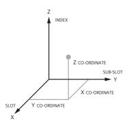
Similar to X and Y and Z co-ordinates on a 3-D map, the information is located at a certain slot, sub-slot, and index. With the map, any-thing in the device can be found.
