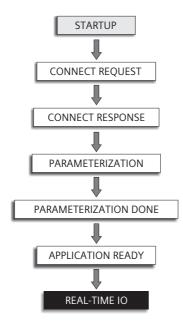
The IO-Controller uses either Discovery and Configuration Protocol (DCP) or Dynamic Host Configuration Protocol (DHCP)<sup>12</sup> to find an IO-Device. Once found it will try to connect to it by sending a *Connect Request*. When it gets a *Response*, it tries to *Parameterize* it, checking several things:
