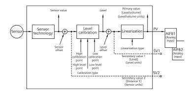
As with subroutines in most computer languages, the values passed between blocks also have a status indicator that indicates that the calculation (or in this case, the process variable) is OK. This status indicator is a logical result of using the block model structure as the blocks can also perform self-diagnostics, alerting the control system to any kind of problem in the instrument itself.
