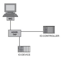
**Passive TAP:** A passive TAP takes the outgoing signal and splits it to one input line in the computer and takes the outgoing signal and splits it to a second input line in the computer. This best solution for IRT covers both performance and data analysis – it's a physical device that would normally be inserted between the IO-Controller and the switch and connected to the two Network Interface Cards (NIC).
