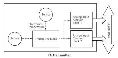
Instrumentation users familiar with HART instruments will use the configuration software and set up the scaling in the transducer block, but will notice the value coming back to the HMI is not correct because with PA devices two blocks need to be set up.
