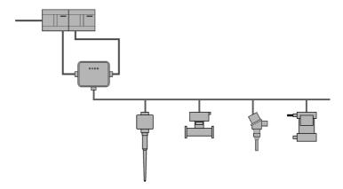
**PROFIBUS PA media redundancy:** Siemens and Moore Hawke both offer PROFIBUS PA media redundancy. The Moore Hawke solution provides only one special junction box in the ring and is therefore limited. This junction box does the switching between the two incoming lines.
