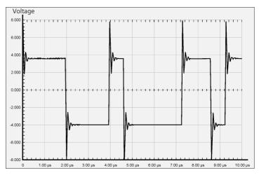
Small PROFIBUS DP network running at 1.5 meg with active terminators turned off and working properly
