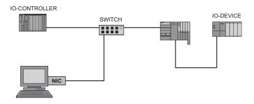
**Aggregating TAP:** A TAP is a Test Access Point. An aggregating TAP combines the input data and the output data (Rx and Tx) from the Ethernet cable into one stream of data going to the input line of the monitoring computer's Ethernet card, called a Network Interface Card (NIC). This physical device would generally be inserted between the IO-Controller and the switch.
