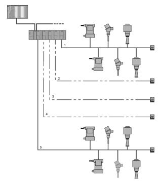
The DP/PA link module is a PROFIBUS slave on the DP side and PROFIBUS master on the PA side, creating a true sub-network. The information in the link module is constantly being updated. As a result, to get all the data to and from the DP master, twice the DP bus scan time is required (at minimum), and the update rate will be:
