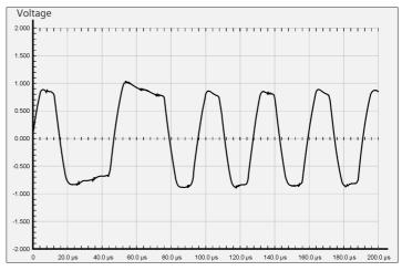
Waveform with one missing terminator
