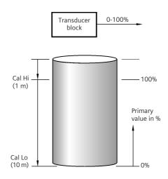
After the calibration block, the value then goes into the linearization block which converts level into volume. This block is defaulted to OFF. Since volume is not required, the defaults are left alone.
