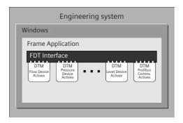
The FDT/DTM solution enjoys a fair bit of success, largely the result of PACTware<sup>™</sup>, a standard software package developed by a consortium of companies, based on the FDT standard, and sharing the source code.
