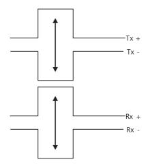
When referring to twisted-pair copper, the nomenclature is xx Base y, the xx refers to the speed in megabits per second and the y refers to the physical layer. In this example of twisted-pair copper, the physical layer is T for twisted pair. For example, 100 Base T refers to 100 megabit per second on twisted-pair copper.
