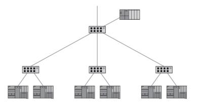
PROFINET is very versatile and can adapt to the application requirements and layout. Basically almost anything works. When laying out a network, the main concern is where best to place the switches and devices. However, keep in mind the effect on the system if a switch fails or a cable is damaged because a failure can drop any number of devices from the network. Also remember that your choice in topology will have an impact on performance as well.<sup>4</sup>
