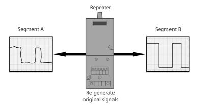
The repeater most common to process automation is the one used for RS-485. Many of these modems will allow as many as nine repeaters in any communication path. Thus between any two devices that talk (master – master / master – slave), there can be no more than nine repeaters; however, the total number of repeaters in the entire system can be much greater than that.
