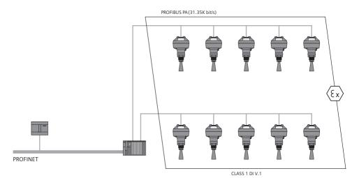
PROCENTEC COMbricks PROFIBUS DP to PROFIBUS PA link/coupler: A transparent solution like the Pepperl+Fuchs power hub product. The DP side can go at any baud rate and there can be up to nine PROFIBUS PA modules in one COMbrick rack. Each PROFIBUS PA module supports one segment. These modules also have the additional option of having a built-in bus monitor called ProfiTrace, one of the leading PROFIBUS bus monitors on the market. Its presence adds troubleshooting options to the system.
