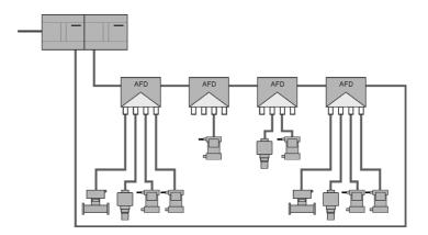
The Siemens solution is to use a ring with multiple junction boxes called Active Field Distributors (AFD). AFD will do the following:
