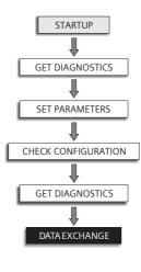
The master then issues a *check configuration* telling the slave what it thinks it is, how many modules the slave has, and how much data it will send and receive. Again the slave will just respond with a short *acknowledge*.
