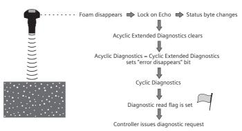
One change in a process condition – such as foam appearing and disappearing – causes two changes in a status byte and two diagnostic requests. Each diagnostic request is logged by the control-
