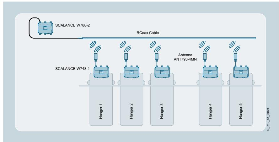
The iPCF IWLAN protocol enables rapid, reliable roaming and deterministic, also failsafe, PROFINET communication in guided, linearly structured applications with RCoax leaky-wave conductors.
