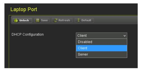
Figure 3-204 CPU III Web UI Site Laptop Port Configuration
