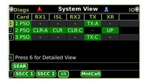
Figure 5-1 Directional Stick Example – Train Not Yet in Approach.
