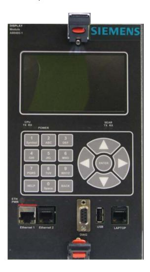
Figure 8-9 Display Module, A80485-1
