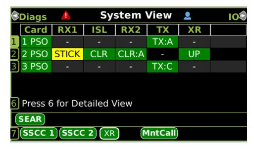
Figure 5-6 Directional Stick Example – Train Exits RX1
