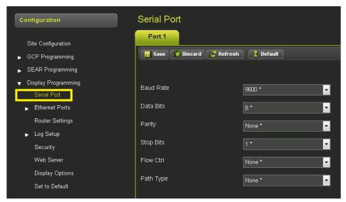
Figure 3-159 Display Programming Serial Port
