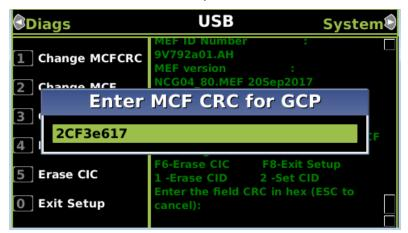
Figure 3-78 Enter MCF CRC for GCP
