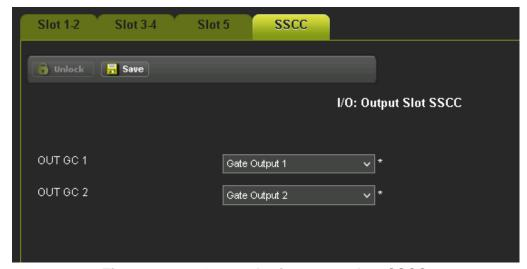
Figure 10-36 Output Assignments slots SSCC
