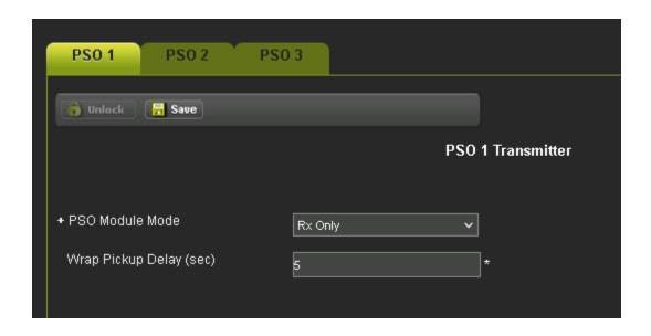
Figure 10-13 PSO Transmitter when mode=Rx Only
