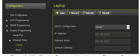
Figure 3-160 Display Programming: Laptop Ethernet Port 3-110
