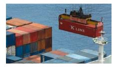
With the semi-automatic mode (SAM) the load is moved smoothly. The load avoids the restricted areas fully automatic with maximum crane dynamics and high accuracy from the start position to the target location.
