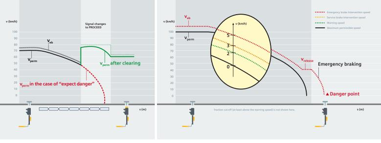
Early acceleration through radio-based clearing
