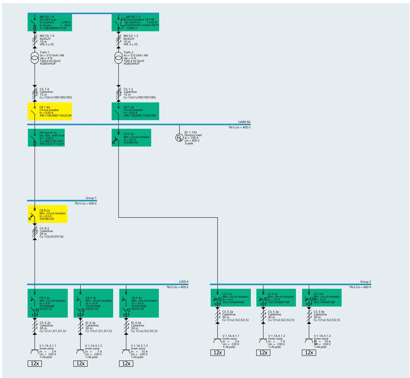
Figure 3: Selectivity evaluation for SHU in SIMARIS design 10 (left, as outgoing feeder to a sub-distribution board and right, as group switch upstream of miniature circuit-breakers; e.g. using MCBs in the range of low-voltage main distribution)
