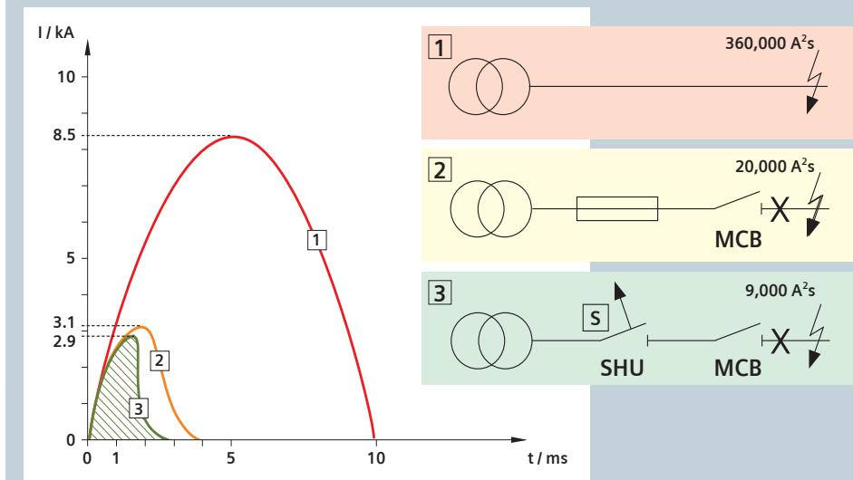
Figure 6: Delayed SHU trip effected by the selective bimetal in case of a short circuit
