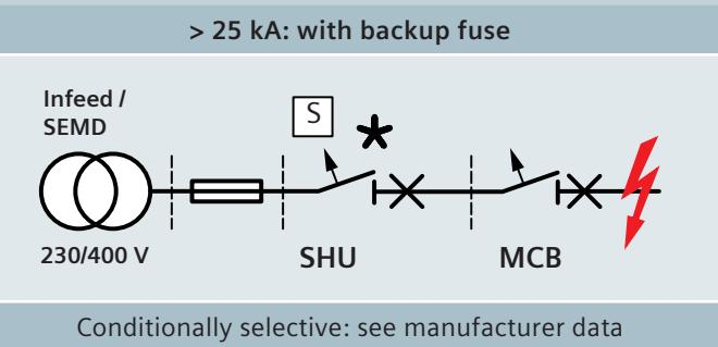
In every combination: fully selective up to  $I_{cn}$  des MCB (6/10 kA)
