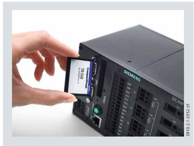
Fig. 4/16 Standard supply: 2 GB CF card (can be upgraded to 16 GB)
