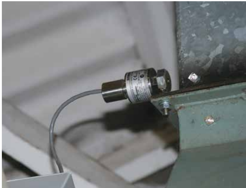
SITRANS AS100 acoustic sensor monitors for a no flow situation in the raw material pipe, alerting operators of any material stoppages.
