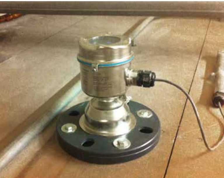
From the raw material storage silos to the dusty midds bins, SITRANS LR560 gives Carr's Flour accurate and reliable level measurement.
