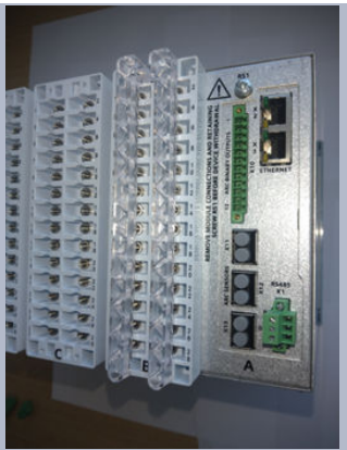
Figure 4.4/4 Terminal block cover fitted to device
