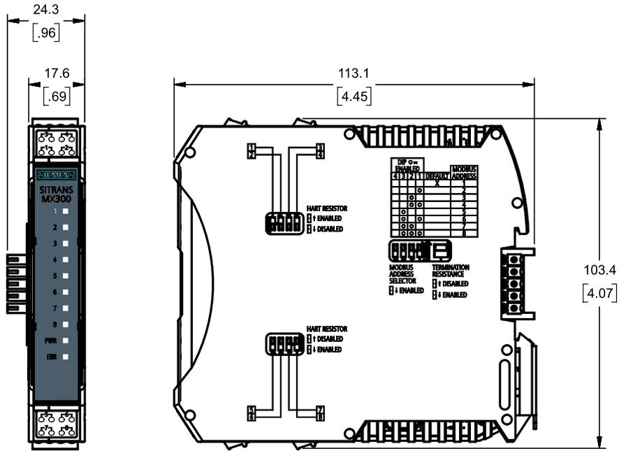
Figure 11-2 Dimension drawings SITRANS MX300, dimensions in mm (inch)
