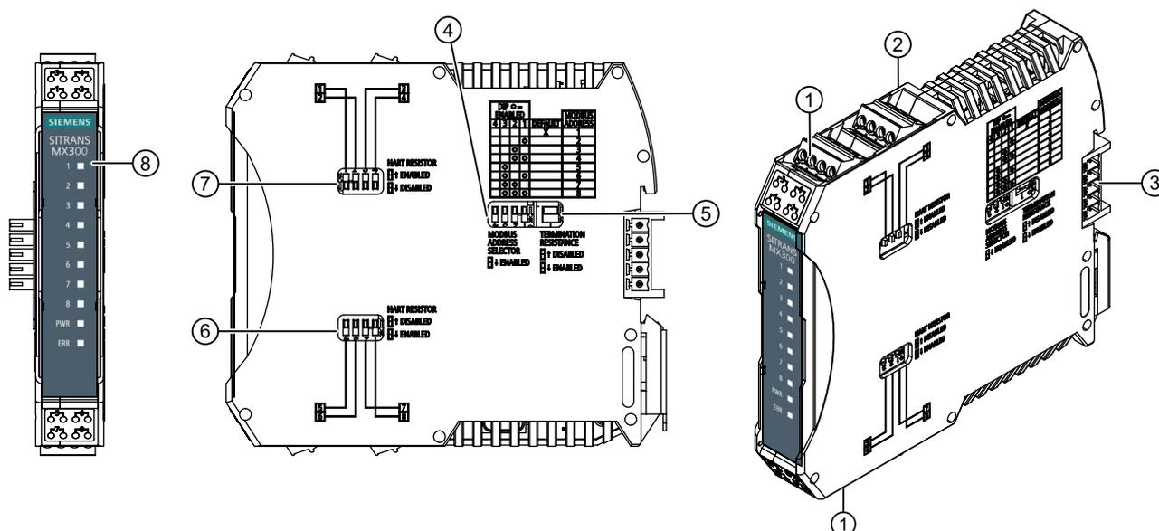
① 1 to 8 Channels for the connection of devices with HART
