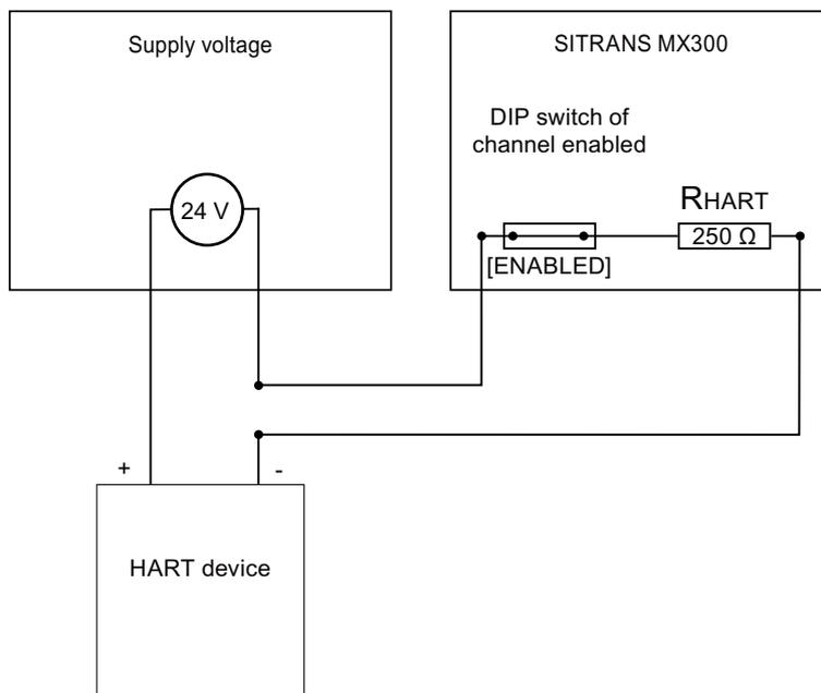
3. Connect one HART device per SITRANS MX300 channel using a two-pole cable.
