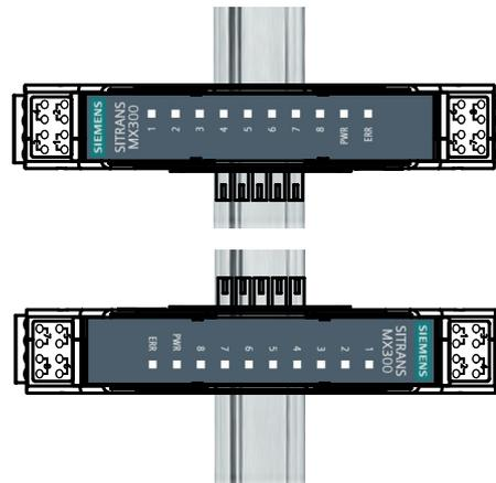
Take into account the permitted temperature range for operation that depends on the mounting position in accordance with the "Technical specifications (Page 67)" section.
