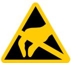
Electrostatic sensitive devices can be labeled with an appropriate symbol.
