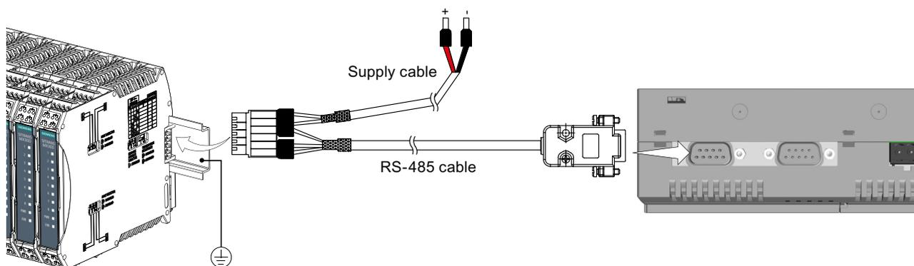
Figure 6-1 RS485 connection MX300 and CC240
