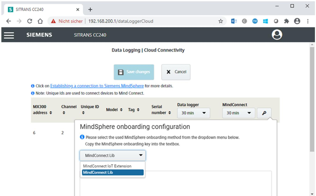
7. Paste the connection key copied from MindSphere into the "MindSphere onboarding configuration" field.
