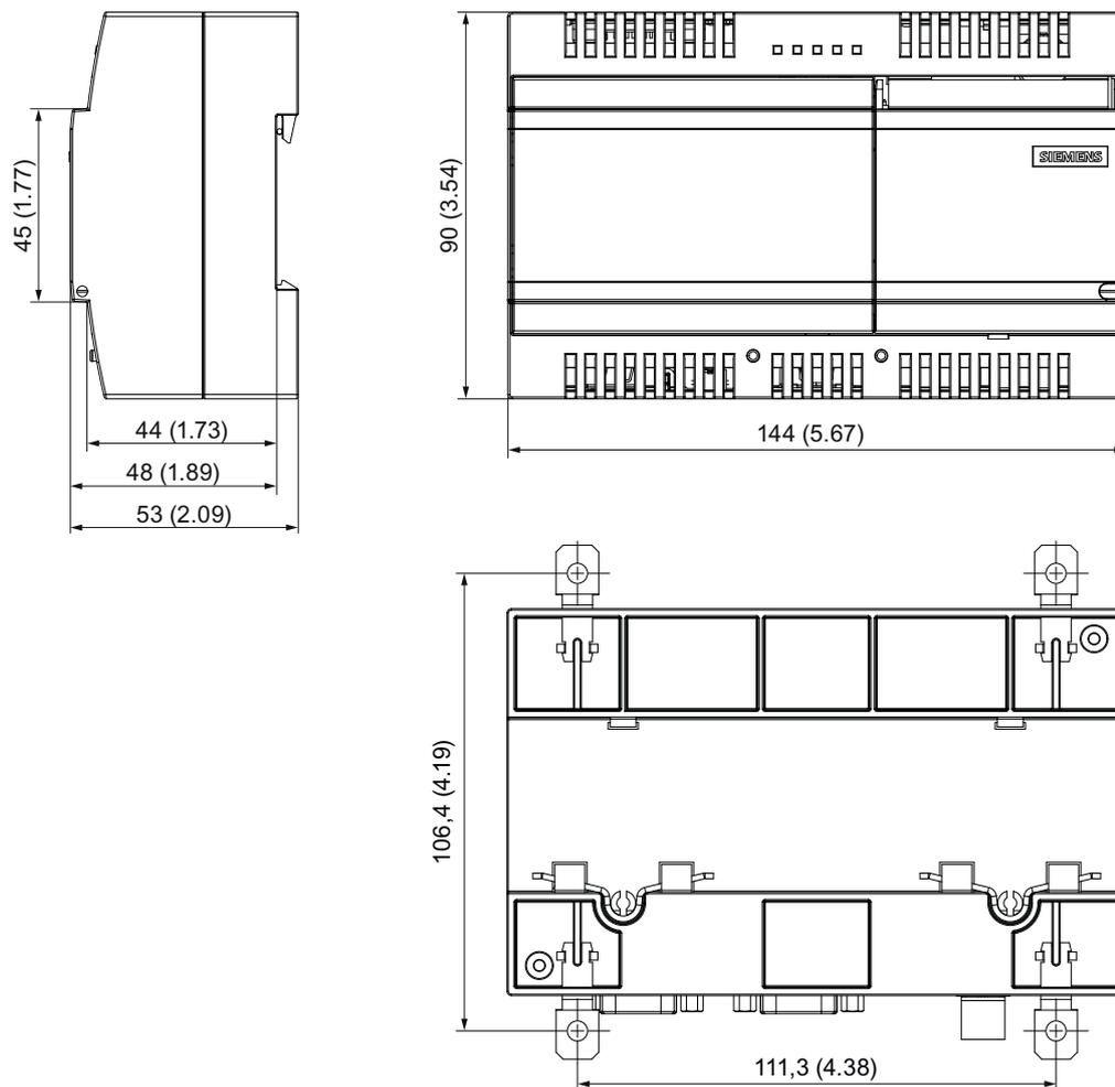
Figure 11-1 Dimension drawings SITRANS CC240, dimensions in mm (inch)
