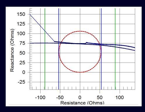
Relay trips on unstable swing on the 2<sup>nd</sup> slip
