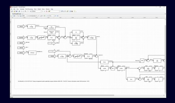
Provides the possibility of creating and testing user-defined models of machine controllers as well as generic network elements (GNE) in a user-friendly, block-oriented environment and of directly using the models without compilation or third-party software in PSS®E. It simplifies enormously the modeling process with regard to modeling itself, model initialization, debugging and documentation.
